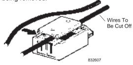
2.04 Precrimp connector with fingers to hold connector and wires in place.
