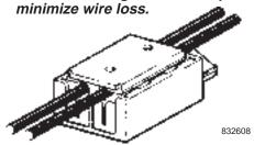
2.05 Crimp connector with Scotchlok™ E-9BM (with jaws set at thick, thick) or E-9E Tool. Wire cut off indicates the connection is made.
